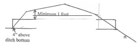
Bottom of culvert intersects with slope.
